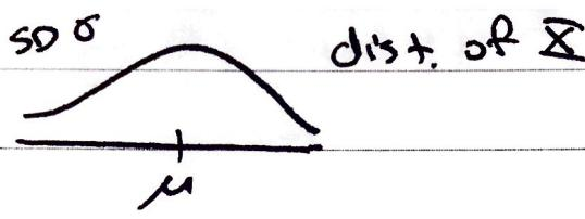
$(\text{center of symmetry, mean, median, mode}) = \text{all } \mu$
